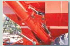
Mechanical auger lock with positive flange seal on 850 and 1075.
