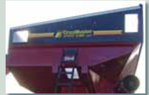
Auger is visible from the tractor cab through the "visibility" cut out of the tank.
