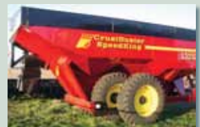
Tandem axle tires go down 30" row spacing.
