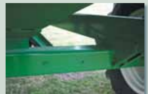
Fully adjustable axle—120" to 144" on 850 and 1075.
